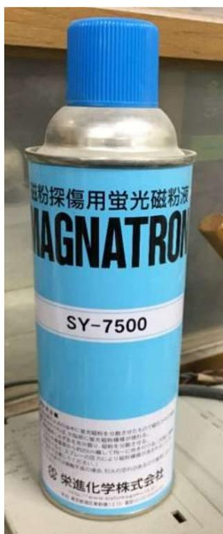
(c) 磁粉探傷用蛍光磁粉液
